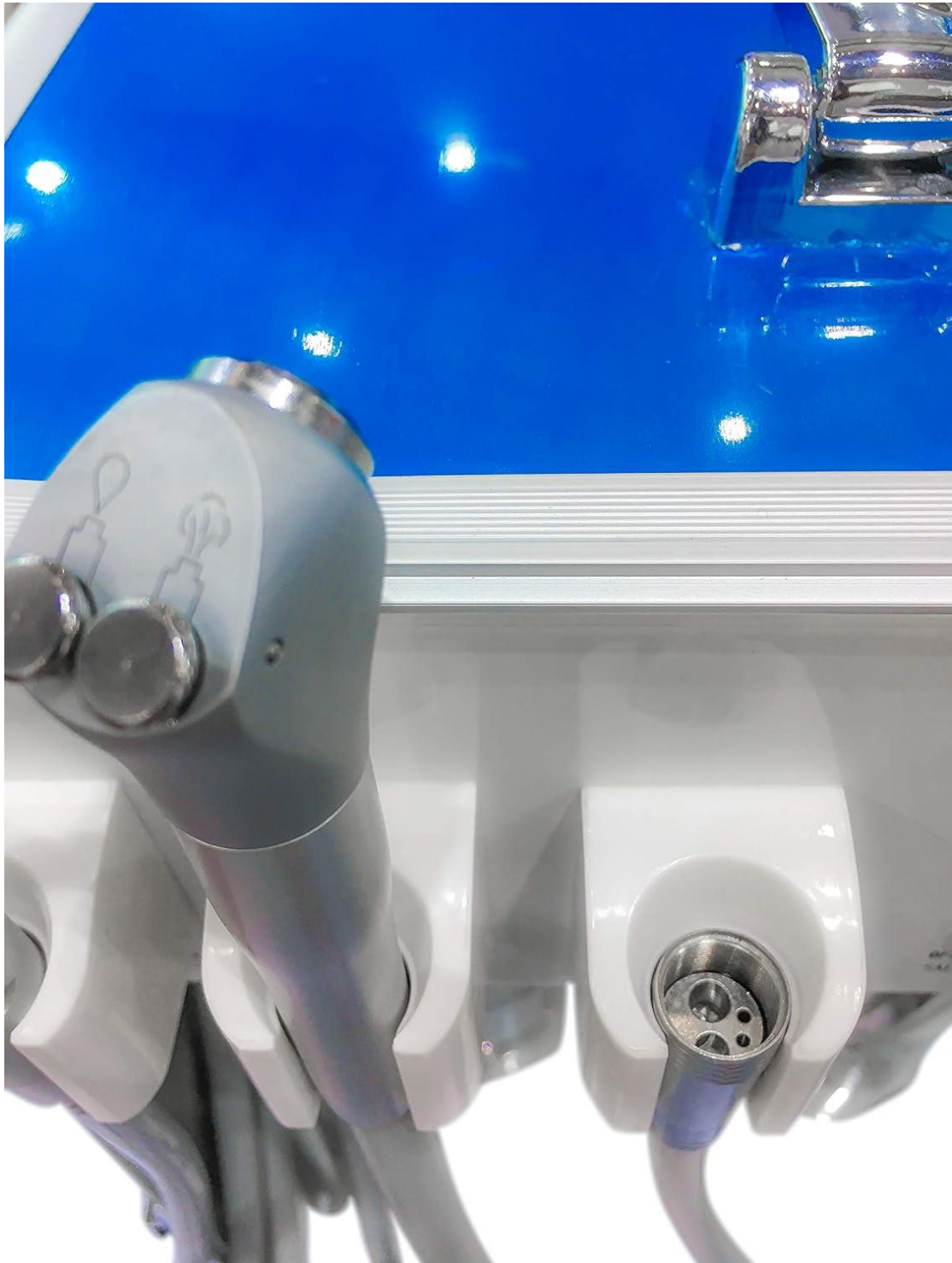
Figure 2: Handpiece Connections. This image shows the connection points for various dental handpieces and hoses, including the high-speed and low-speed air lines.
