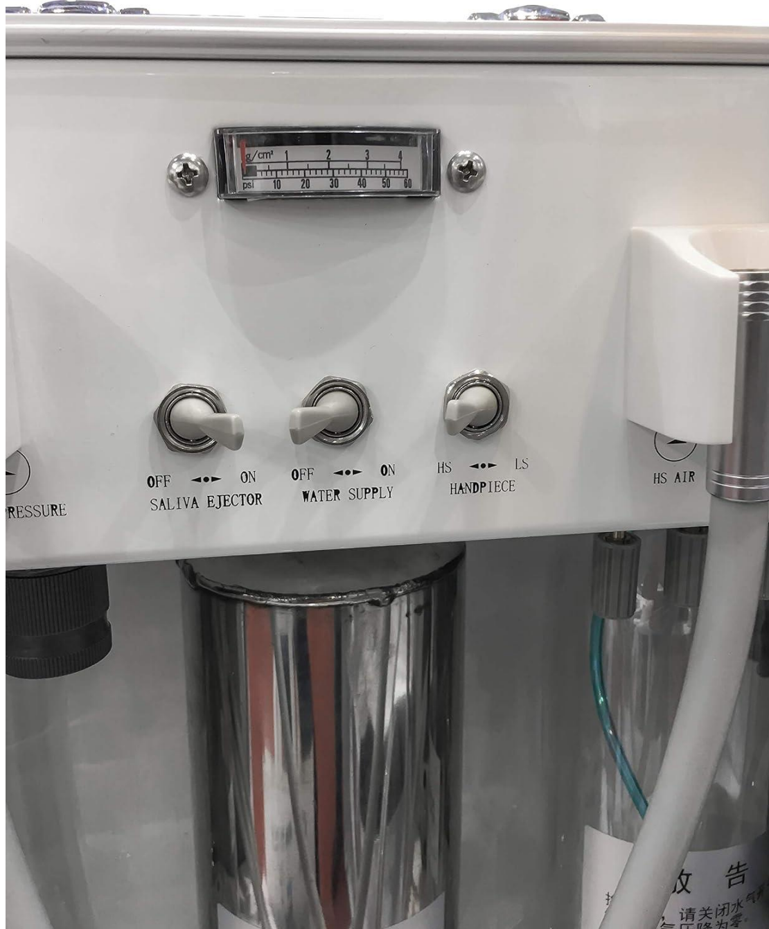
Figure 4: Control Panel. This image provides a close-up view of the unit's control panel, featuring a pressure gauge and toggle switches for Saliva Ejector, Water Supply, and Handpiece (HS/LS) activation.
